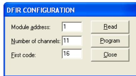
Enter in the first text box the starting address that was assigned to the module (e.g. 1) and then press the Read button. The window will show the current configuration of the module in the other two text boxes; in the case of factory configuration, the boxes will show “Number of channels = 11” and “First code = 16” as in the previous figure.
