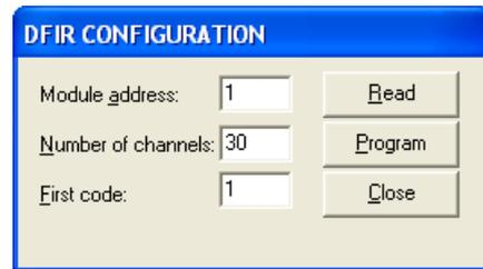
Press then the Program button to send the new configuration to the module. This one, for the configuration shown in this example, will take one address for the two physical inputs (terminal 3 and 4) in addition to an amount of addresses given by the greater integer of:
