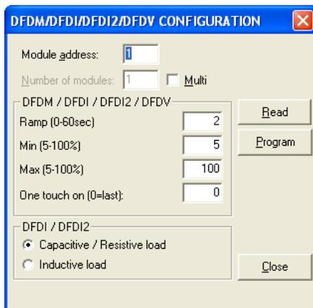
Enter in the related text box the address of DFDI2 module to be set and the ramp value, then click on Program button. Clicking on the Read button, it is possible to check the current setting of the module.
