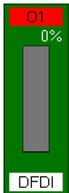
The bar graph shows the output level of the module, and the number over the bar shows the same value in numerical format. To change the output level, click on the bar graph using the left button of the mouse, enter the desired value and then confirm it by the Enter button on the keyboard.
