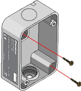
Introduce the bus through the cable bushing: pay attention to the coupling between them in order to assure the waterproof characteristic of the module. After that connect the bus cable to the 2-way removable terminal block: pay attention to the polarity.
