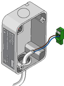
Finally, insert the removable terminal block into the related male connector. Place in the correct way the gasket on the cover and apply to the bottom of the module: pay attention that the removable terminal block be on the opposite side of the cable bushing.
