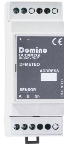
The meteorological station has a 5-way removable terminal block with a premounted diode for reverse polarity protection; however, pay attention to the connection of the meteorological station because, in the opposite case, it could be irreversibly damaged. The connections must be executed before to apply the power supply.
