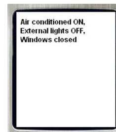
➤ **Messages from user to DFGSMIII for command execution or information request:** Each SMS message sent by the user to DFGSMIII module may contain one or more commands; the commands can act on the local outputs of the module or on one or more of the 64 fictitious inputs provided by DFGSMIII (remember that the module is seen by the bus as an input module with 4 addresses, 16 points each one; these inputs must be used in the **Domino** equations to perform the desired actions).
