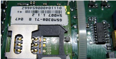
Under the front panel is also located a jumper allowing to connect/disconnect the Li-Ion battery. To avoid the battery discharge, the module is provided with the jumper unplugged; the installer, during the setting up, has to plug the jumper as in the following figure.
