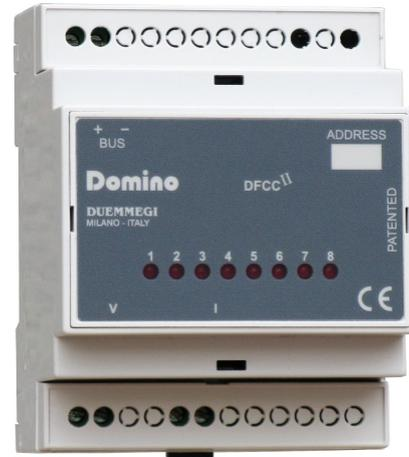
If a power overload occurs, the first load to be disconnected will be the number 8 (which must be that considered the less important by the user). The load shedding occurs after 2 seconds after exceeding the threshold; in this case, if there still remains the overload condition, DFCC2 module will disconnect the successive loads until the total power returns below the thresholds.
