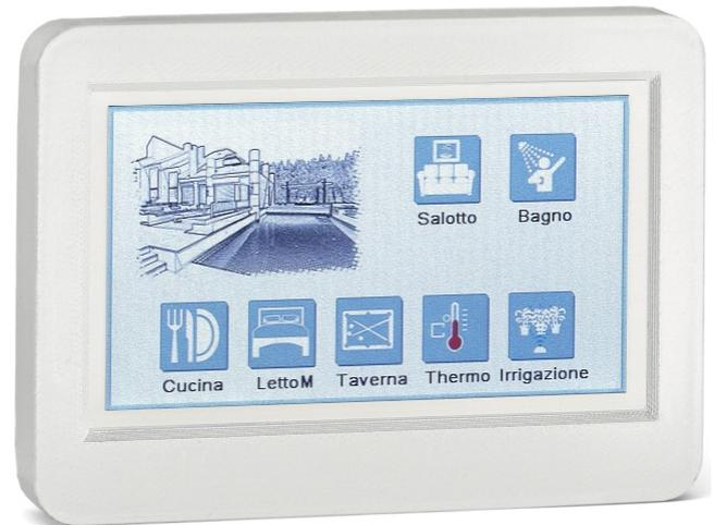
A single DFPW2 power supply, in a **Domino** system, can supply up to about 50 "generic" modules (in other words the classic input and output modules of **Domino** family). DFTouch2 video terminal has a "weight", in terms of current consumption, equal to 18 generic modules; therefore, take in account this data when designing the plant, in order to install the correct number of DFPW2 modules.
