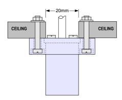
Insert the cylinder of the sensor in the provided ring, from the side where the hole is bigger. Fix then the ring and the sensor to the ceiling by 2 screws with nuts or by 2 Parker screws.
